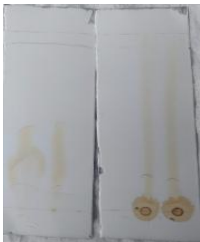
Figure 1. TLC spots on n-hexane:methanol 9:1 eluent (left) and diluted extract (right)
