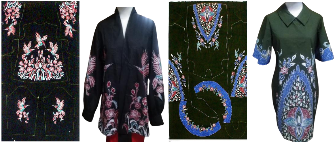
Figure 9. Indicate the alignment of motif shape, motif size, motif positioning, and placement of the motif according to the fabric grain direction, as well as the efficiency in material usage (spacing between pattern sections) (Source: Personal collection)
